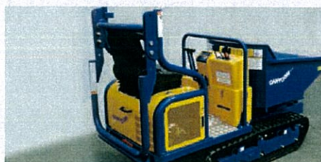
Folding ROPS For transport and job site with limited height
