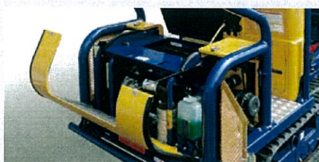
Wide opening covers For an easy access to E/G components
